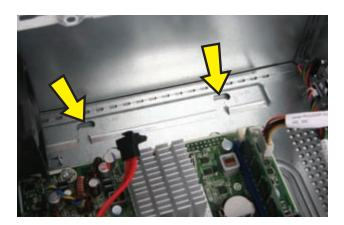
Push the hard drive back into the bay and then to the right until it locks. When the drive is properly located, the threaded holes in the drive line up with the holes in the drive bay, and the power and data cables will route properly.
